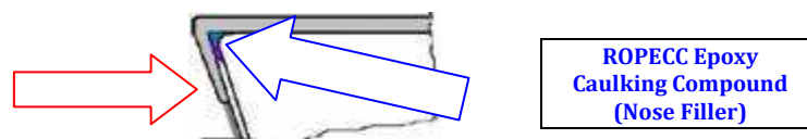
Adhering Stair Treads Nosing to Riser with ROPECC Epoxy Caulking Compound
